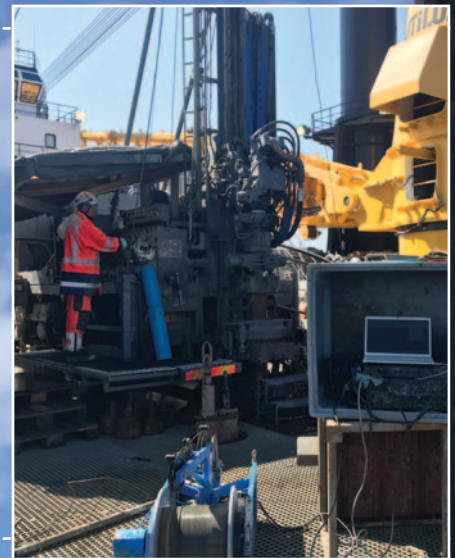
Robertson Geo's 2,000m marine winch secured to the drilling deck with the PS Logger laid out to its left and ready to be deployed.
