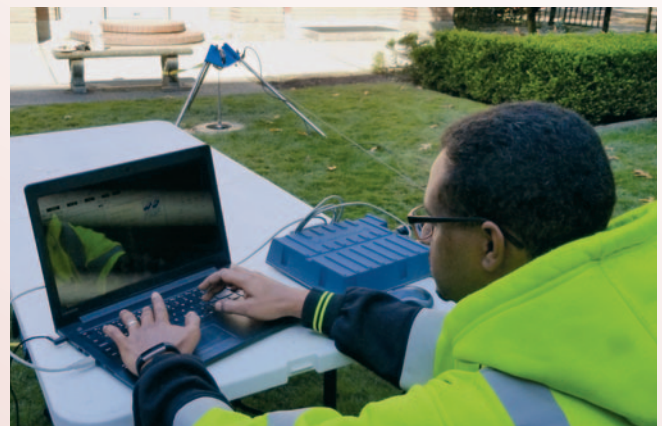
Mr. Meron Okbay MS of Insitu Engineering accessing data from the PS Logger deployed into the pilot borehole at Trinity Parish Church.
